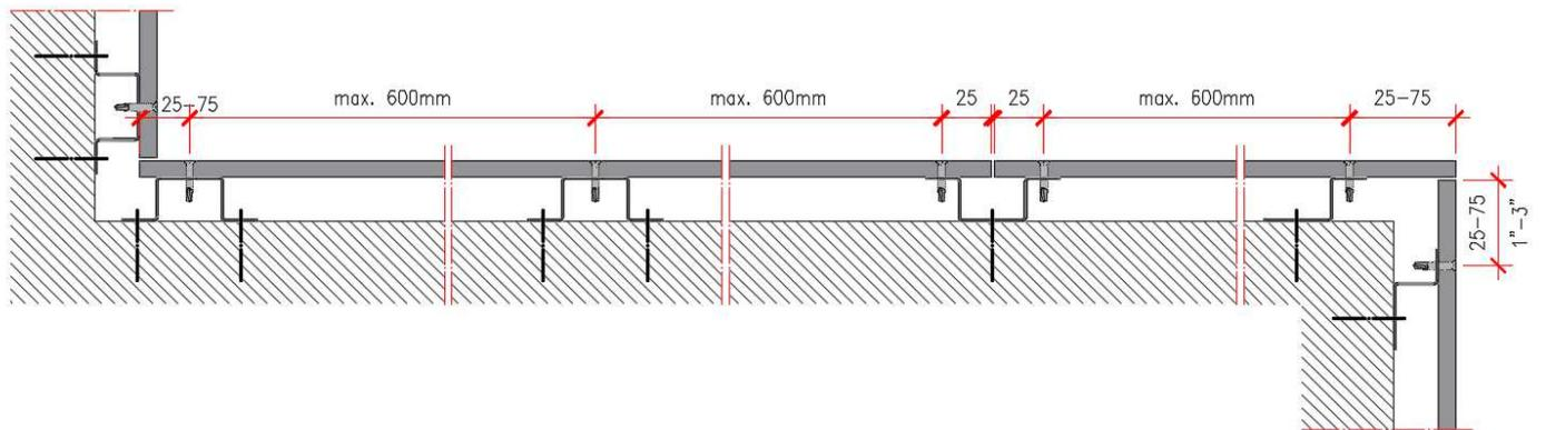
Figure 2.22 - Horizontal section, galvanized steel structure
