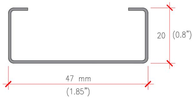
Figure 4.4 - C profile, galvanized steel Dx51D (Z+)
