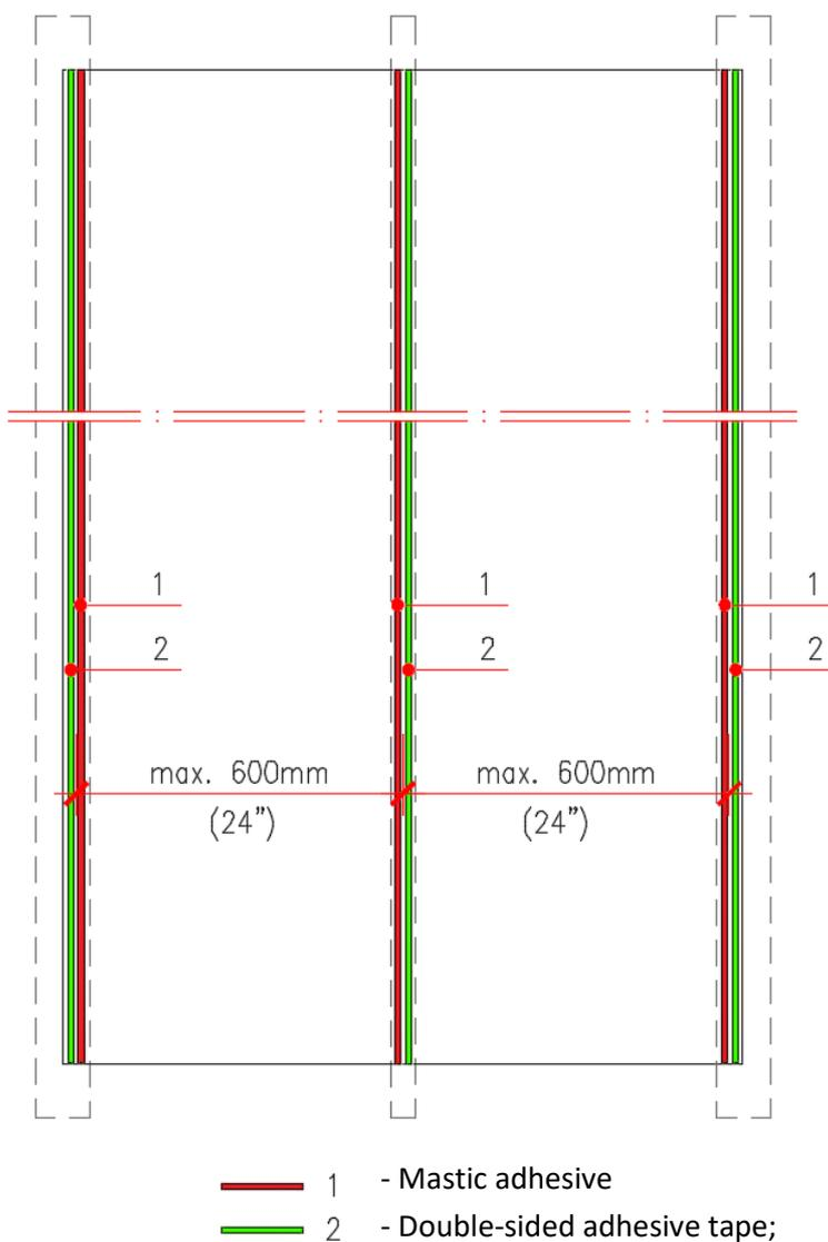
Figure 2.2 - Gluing system location
