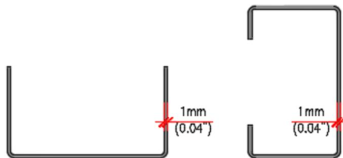
Figure 2.13 - Section type of structure in galvanized steel (Channel)
