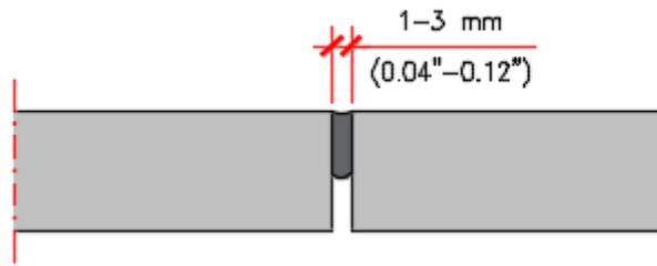
Figure 2.25 - Joints between panels with mastic filler
