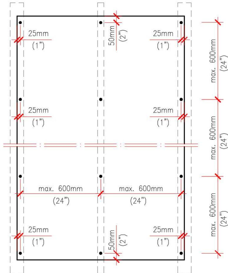
Figure 2.5 - Screws/rivets location
