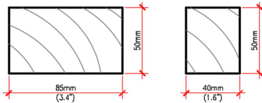
Figure 2.12 - Section type of wooden structure
