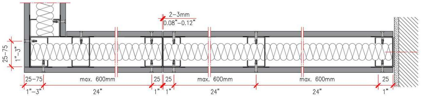
Figure 2.17 - Horizontal section of the wall, galvanized steel structure
