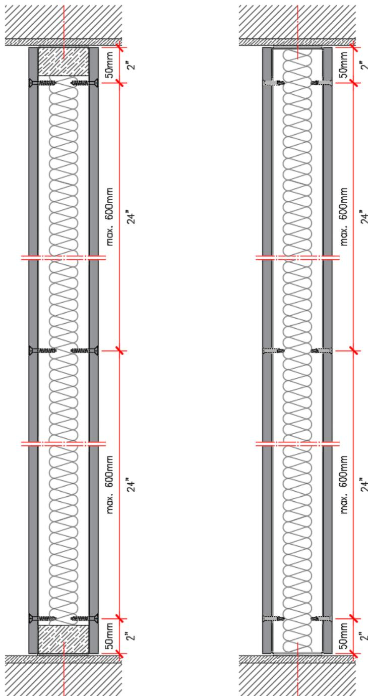
Figure 2.18 - Vertical section of the wall
