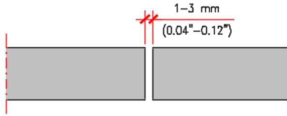
Figure 2.24 - Joints between panels
