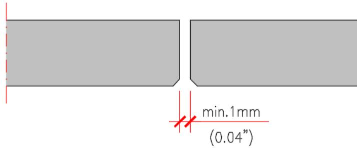
Figure 4.9 – Bevelled edge
